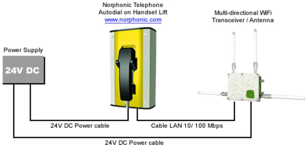
The flexibility of the Norphonic Emergency Roadside Telephone therefore means that it could be used on a fixed fiber cable layout or in a wireless VoIP environment. There are no particular barriers to installing Wireless / WiFi Emergency Roadside Telephone solutions, but the network designer should be aware of potential voice quality pit-falls and plan for these.
