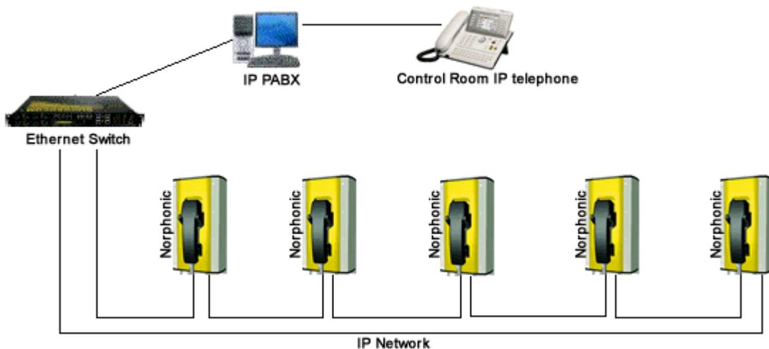
(Each Norphonic telephone have two integrated Fiber Optic Ports - Single Mode, 100 Mbit)
