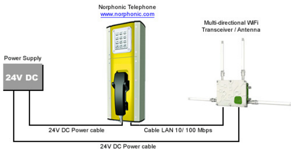
Fig 3: Example of a Norphonic telephone connected to a multi-directional transceiver / antenna to facilitate Wireless / WiFi communication in offshore / maritime areas, on board ships etc.
